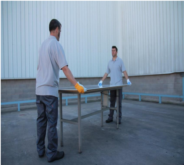
Surface of the working bench should be completely flat and clean before placing the sheet on top.
